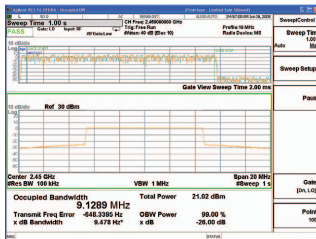
Figure 32. Frequency error reported along with occupied bandwidth measurement on MXA
